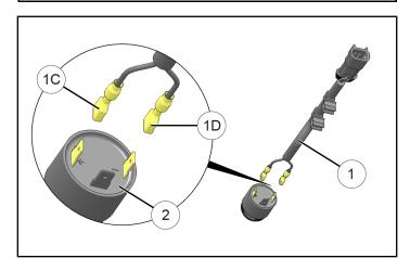
4. Remove knurled nut from reverse beeper ②, install beeper rearward through hole in bracket ③, then reinstall and tighten knurled nut.
