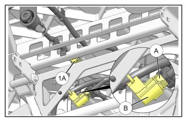
Slowly raise vehicle bed to ensure harness routing does not allow contact with hot components, sharp edges, or moving parts. If so, adjust routing and/or secure harnesses as required.
