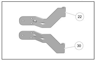
d. Loosely install LH lower door-side hinge ② to FRONT LH door using three each carriage bolts © and nuts ①.
