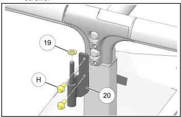
j. Install nylon washer (9) to hinge pin.
