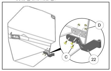
4. Install chassis-side hinges for **FRONT** door.
