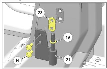
g. Install nylon washer 19 to hinge pin.
