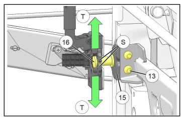
c. **DEPTH** ①: As required to achieve desired seal compression and door fairing. To adjust, loosen nut ®, slide striker pin ⑥ inboard or outboard as required, then retighten nut.
