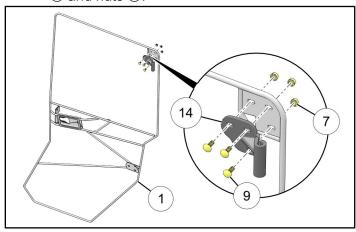
c. Identify **LH** lower door-side hinge **3**. Notice differences from **RH** lower door-side hinge **3** (especially angle of joggle ①).
