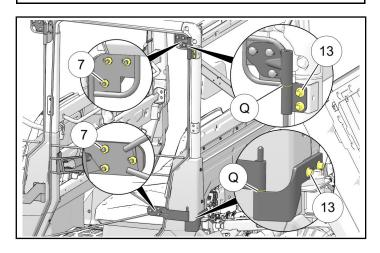
9. Torque all four chassis-side hinge screws ③ and all six door-side hinge nuts ⑦ to specification.
