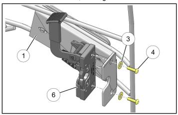
14. Open door latch (to properly position pawls), then slowly close door and observe engagement of striker pin (6) into door latch.
