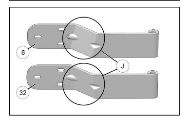
d. Loosely install LH lower door-side hinge ® to LH rear door ① using three each carriage bolts
