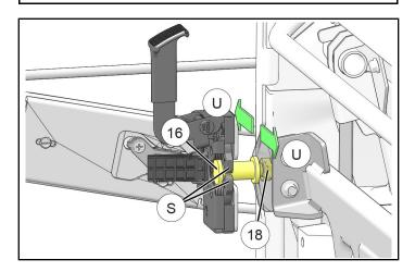
15. Torque striker bracket screws <sup>(3)</sup> to specification.
