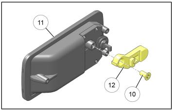
12. Install exterior latch ① to LH door frame ① using three screws ③. Center latch in slotted holes, then tighten screws.
