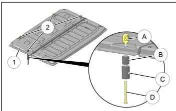
3. Assemble REAR anchor ③ as shown. Repeat for second anchor.
