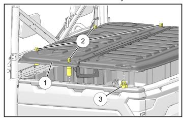
6. Tighten handles on four FRONT anchors ② until anchors are secure.
