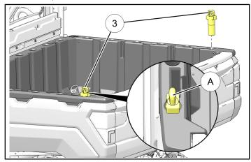
5. Install tonneau cover ① to vehicle bed, inserting four front anchors ② into corresponding holes in vehicle bed until anchors are fully seated.
