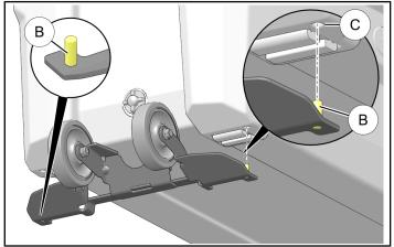
4. Install two locking screws (6) through sides of frame/wheel assembly into mating holes (A) on cooler. See Step 2.
