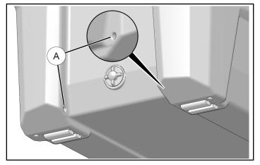
3. Install frame/wheel assembly to DRAIN end of cooler by fully inserting two pins <sup>®</sup> into mating holes <sup>©</sup> on bottom of cooler.
