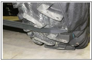
e. Tension strap sufficiently to prevent it from slipping above tire lugs during transport, then fully close ratchet lever (A).
