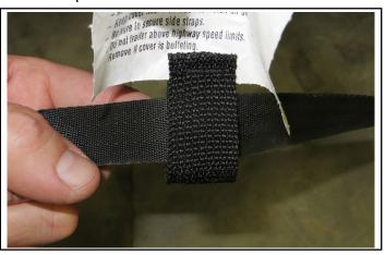
c. Pull RH strap tight, then fold strap and insert into ratchet (A) spool.
