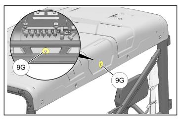
b. From outside cab use 1.25 in (32 mm) hole saw, centered on pilot hole, to drill forward through roof panel.
