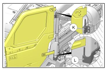
c. Remove UPPER chassis-side hinge ( by removing two screws ( and nut plate ( ). Retain hinge (with nylon washer). Screws, nut plate, and conical spring washers (if installed) will not be reused.
