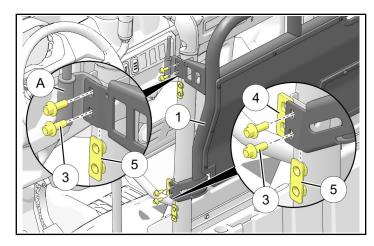
2. Loosely install LOWER LH corner of frame ① to ROPS using two screws ③, spacer ④, and nut plate ⑤.
