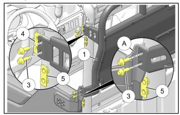
2. Loosely install LOWER LH corner of frame ① to ROPS using two screws ③, LH door assembly (with upper chassis-side hinge ⓐ), and NEW nut plate ⑤. Spacer ④ is not used.
