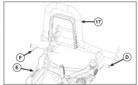
**NOTE:** Make sure the hook up (17) can move as shown in the picture. If this is not the case, remove the clevis pins (D) and reposition the handle so the stops function correctly.
