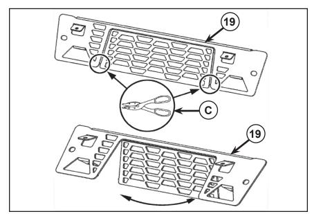
7. Install the new grille (19) to vehicle using the existing bolts removed in step 6.
