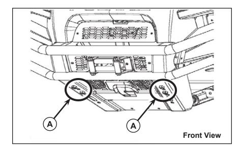
2. Fasten the upper part of the mount plate (9) to frame using the four M12-1.75 X 30 mm hex bolts (5) and four M12-1.75 nyloc nuts (7) (finger tighten at this time).
