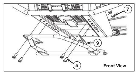
3. Fasten the lower part of the mount plate (9) to frame using the three M10-1.5 X 35 mm hex bolts (4) and three M10 lock washers (20), and the threaded support (10). Tighten all bolts and nuts.
