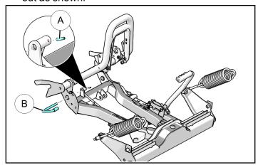
2. Insert new kick stand rod ① into place and secure with pin ⓐ previously removed. You will need to align the holes in the kick stand rod and kick stand rod sleeve ⓒ.
