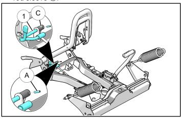
3. Install the new lift link ② between the winch (not shown) and the plow frame assembly ⑩ instead of the link originally included with kit 2881286 by placing into position as shown and securing with the winch link pin ⑥ and cotter pin ⑥ provided with kit 2881286.
