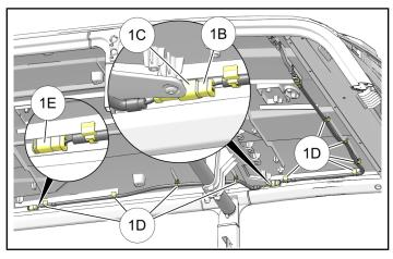
5. Secure extension harness ① to roof using five edge clips 1D on front harness segment, and if installing on crew vehicles, four additional edge clips 1D on rear harness segment.
