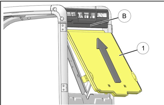
4. While keeping upper edge of panel ① on FORWARD side of ROPS cross member (B), tilt lower edge of panel forward. Slip both panel brackets (C) over cab cross member (D), then lower panel until brackets are fully engaged. Ensure panel is centered from right to left.
