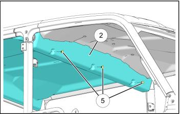
Install rear headliner (2) to roof panel using four push darts (5) and two each screws (4) and washers (3). Torque screws to specification.
