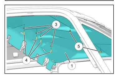
Raise rear headliner 2 into position, inserting tabs on front edge into corresponding slots on rear edge of front headliner 1. Secure to roof panel using three push darts 5.
