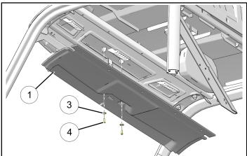
4. Insert both rear segments ① of rear liner ② into roof support channel, then slowly tip liner up, inserting LH and RH edges of liner between ROPS and roof seal.
