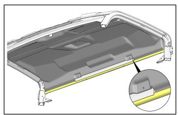
5. If installing optional light, then refer to instructions included with light. Otherwise, install two each screws 4 and washers 3 through rear liner 2 into roof.
