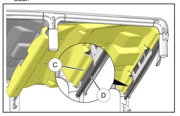
If installing optional light, then refer to instructions included with light. Otherwise, loosely install two each screws (4) and washers (5) through rear liner (1) into roof.
