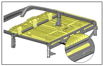
2. Hold front panel ② at slight angle above ROPS as shown. Insert rear edge of front panel ② into channel on front edge of rear panel ①.
