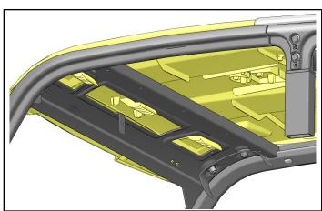
4. Secure rear panel ① to front panel ② using eight screws ⑤.
