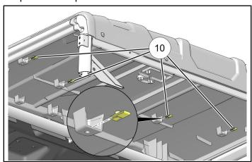
6. Insert rear edges © of rear liner ① into roof support channel ⑩, then tip liner up, inserting LH and RH sides of liner between ROPS and roof seal.
