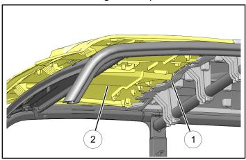
3. Lower front of panel ②, inserting three hooks ⑤ through openings in ROPS visor ⑥, then slide panel rearward until hooks lock into visor.
