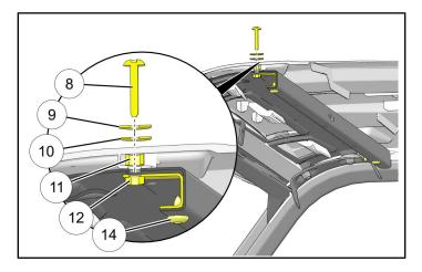
7. Torque screws to specification (as applicable to your kit).
