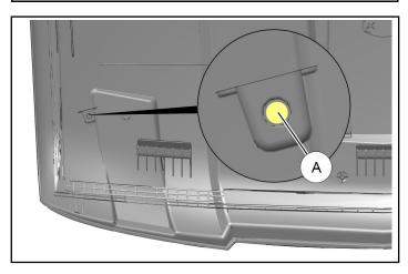
b. Insert spacer ① into each standoff. Use tape to prevent spacer from falling out of standoff during roof installation.
