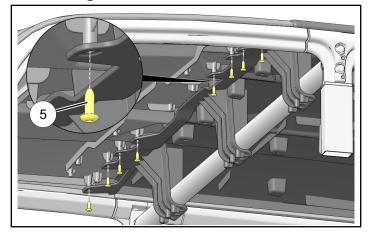
5. Secure rear panel ① to C-pillar cross member © using four screws ⑥.
