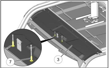
4. If installing optional light, then refer to instructions included with light. Otherwise, loosely install two each screws ④ and washers ⑤ through mid liner
