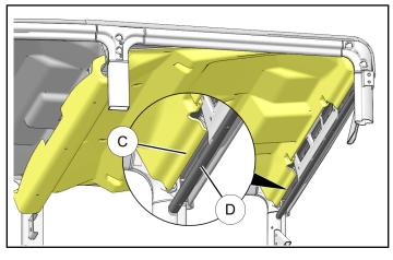
If installing optional light, then refer to instructions included with light. Otherwise, loosely install two each screws (4) and washers (5) through rear liner (1) into roof.
