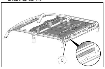
3. Install rearward edge of front roof panel ② into channel on frontward edge of rear roof panel ①.
