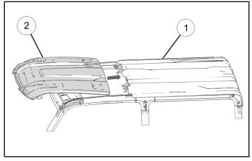
4. Install hooks on front roof panel ② through openings in ROPS visor. Move roof panel rearward until hooks lock into visor.
