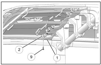
2. Attach rear roof panel ① to C-pillar cross member ② using four screws ⑩. Torque to specification.
