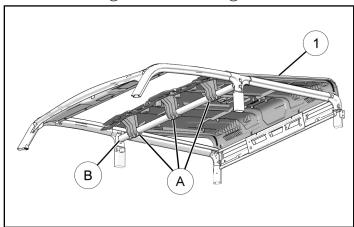
2. Install two rearward roof panel tabs into C-pillar cross member ©.
