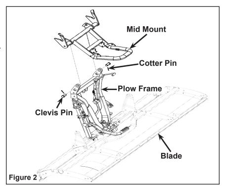
3. Feed the top of the mid mount to the inside of the track extension between the top mounting locations and secure the lower mounts to the track extension (PN 2879871) using the two M20X50 mm bolts and nylock nuts. Figure 3. Leave hardware finger tight at this time.
