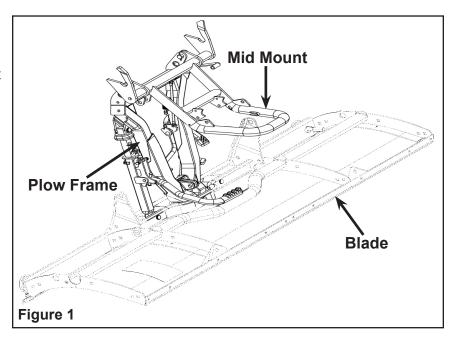
2. Remove the two cotter pins and clevis pins securing the mid mount to the plow frame. Remove the mid mount from plow frame at this time. Retain the hardware for reuse. Figure 2.
