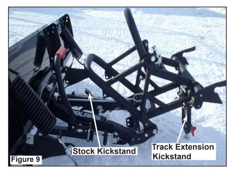
The track extension kickstand does not retract automatically. Use the foot actuated kickstand release lever shown in Figure 10 to release the kickstand once the system is securely latched to the machine.
