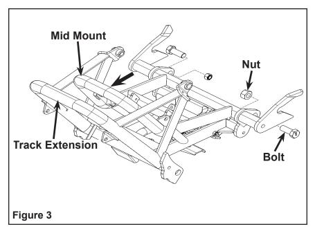
4. Rotate the mid mount rearward to align the top mounting locations of the mid mount with the top mounting locations on the track extension. Figure 4. Secure the mid mount in place using the two M12X50 mm bolts, washers and nuts provided in this kit. Torque hardware to 50-60 ft. lbs. (67-81 Nm).
