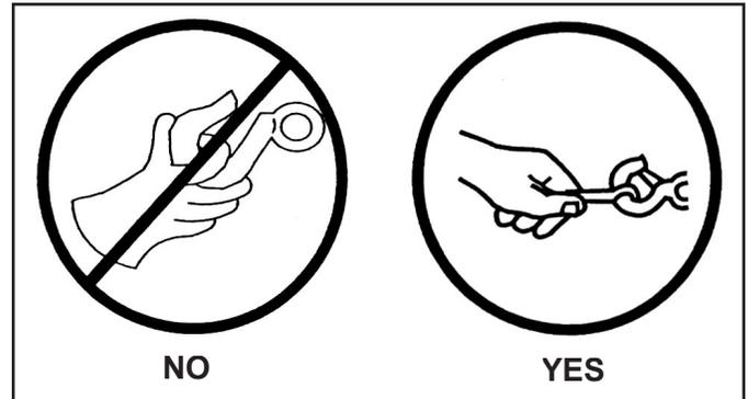
**WARNING! Never use a recovery strap when winching due to the excessive energy that can be released if the winch cable breaks. This can result in SEVERE INJURY or DEATH. See the Shock Loading section on page 6.**
