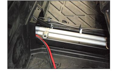
2. Slide the other end of cable through bulkhead. Follow main wire harness up and onto the splash tray as shown in figure.
