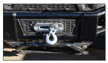
7. Reinstall front bumper with fastener removed earlier. Make sure the winch cable or rope is through the fairlead slot as shown in figure.
