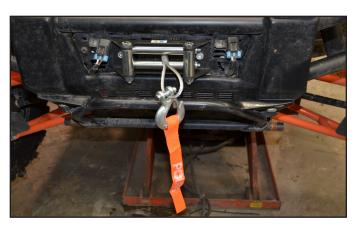
8. Connect the yellow and blue winch wires to contactor and push cable covers on as shown in figure.
