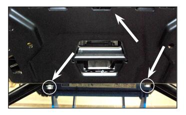
3. Line up holes in front of machine to mount winch.
