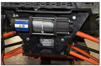
Connect yellow and blue cables to the corresponding post on winch with a 10 mm wrench. Push cables up through the splash tray and to contactor as shown in figure.
