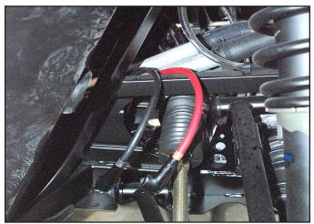
3. Connect short (250 mm) red and black cables to the bus bar on the same posts as the wires previously connected. Reinstall nuts on bus bar. Connect wires to red and black terminals on contactor and lightly tighten. DO NOT OVER TIGHTEN. Slide the cable covers on as shown in figure.
