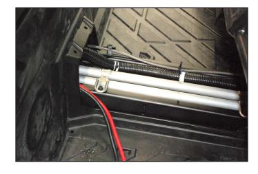
2. Slide the other end of cable through bulkhead. Follow main wire harness up and onto the splash tray as shown in figure.
