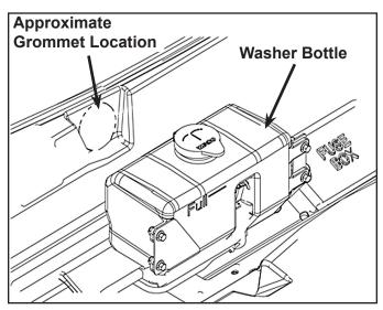
5. Push the wires back through the grommet and replace grommet in upper splash tray hole. Connect black wire to connector and red wire to the keyed power terminal. After wires are connected, panduit power and ground cables to the main wire harness to keep clear of moving parts and panduit to frame as shown in figure.
