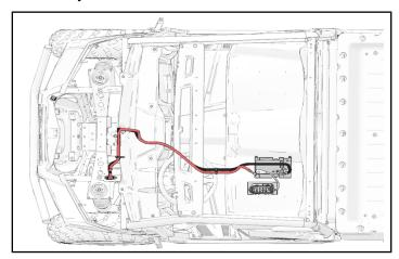
4. Double-check wire routing to make sure red and black cables are secured away from any moving or potentially hot parts. Reinstall center floor.
