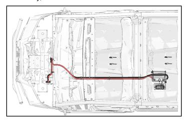
4. Double-check wire routing to make sure the red and black cables are secured away from any moving or potentially hot parts. Reinstall center floor.
