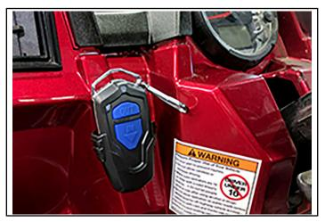
b. Using holder (2) as template, mark and drill two 1/8 inch (3 mm) holes into mounting surface.
