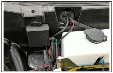
b. Join connector on wireless receiver (2) to mating connector on Y-splitter harness (2).
