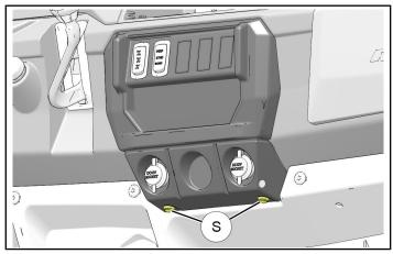
b. Rotate bottom of control panel rearward, disengaging two side tabs ①, then drop two upper tabs ① out of slots in main dash panel.
