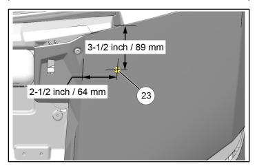
e. Disassemble nozzle ②, then loosely install to fender.
