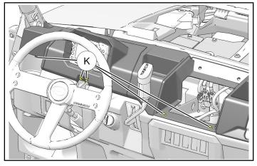
e. Open door to upper storage compartment. Remove three push pin rivets ① from RH side of dash: two inside storage compartment and one on underside of dash above cupholder.
