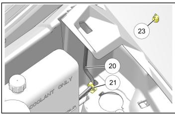
g. Secure washer bottle hose @ and power harness ® to underhood liner using two edge clips ②. See previous Steps c. and f. for location of edge clips.
