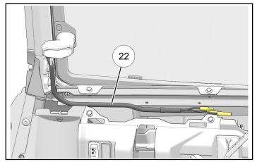
b. **MATCHING WIRE COLORS**, join bullet connectors 22A–22D on ROPS harness ② to mating bullet connectors 18G–18K on power harness ®.
