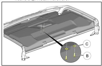
d. Carefully pull LH and RH edges of rear liner from between ROPS and roof seal, then remove rear edge of liner from roof support channel ①.
