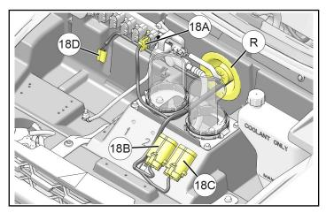
b. Drill out two accessory plugs (1/4 inch / 6 mm) on under-hood liner, just forward of air intake ducts, then install relay blocks 18B and 18C using attached fir tree clips.
