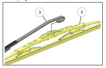
h. Lift arm cover @. Orient wiper blade/arm assembly parallel to top of windshield, then install to wiper motor shaft N. Install washer 8 and nut 7.
