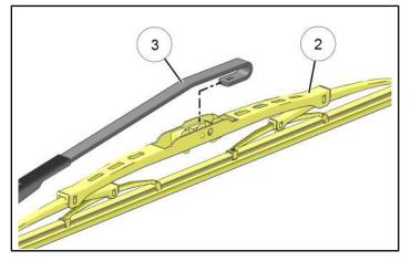
h. Lift arm cover (1). Orient wiper blade/arm assembly parallel to top of windshield, then install to wiper motor shaft (1). Install washer (8) and nut (7).
