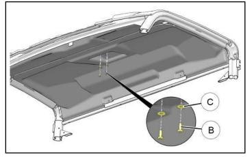
d. Carefully pull LH and RH edges of rear liner from between ROPS and roof seal, then remove rear edge of liner from roof support channel <sup>(1)</sup>.
