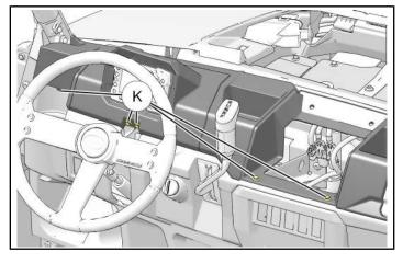
e. Open door to upper storage compartment. Remove three push pin rivets ① from RH side of dash: two inside storage compartment and one on underside of dash above cupholder.
