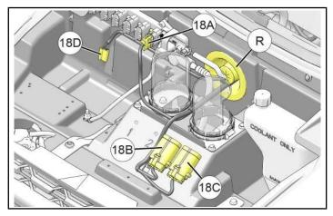
b. Drill out two accessory plugs (1/4 inch / 6 mm) on under-hood liner, just forward of air intake ducts, then install relay blocks 18B and 18C using attached fir tree clips.
