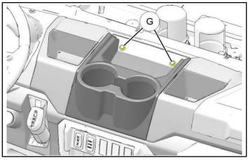
c. Remove six push pin rivets ① along forward edge of dash.
