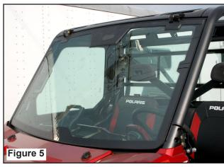
7. Install bolts through windshield hinges to holes provided on vehicle frame. To allow for adjustments, snug just one bolt each side. Open and close the windshield a couple of time to make sure it is centered on vehicle. Once this is accomplished, torque bolts to 20 ft. lbs. (27 Nm). Figure 6.
