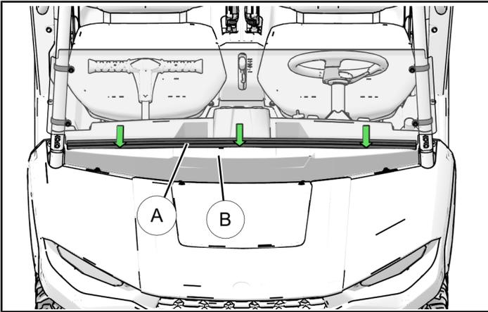
5. Once windshield is in the proper position, torque mounting fasteners (5) on all four corners of windshield to specification provided.
