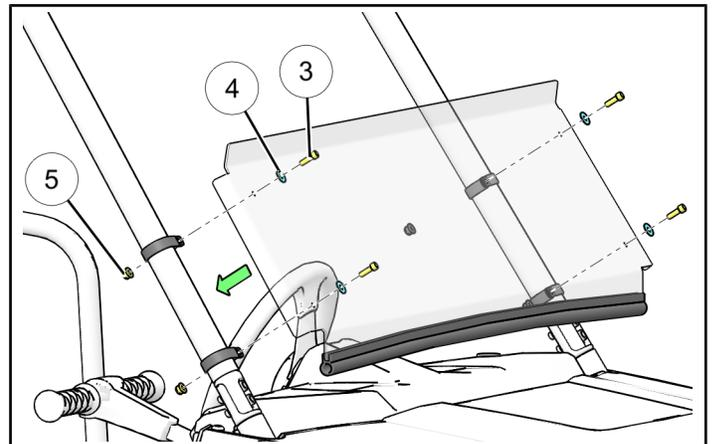
4. After installing and BEFORE TIGHTENING the mounting hardware, firmly pull the windshield downward to ensure the rubber gasket (A) comes in contact with the upper dash panel (B).
