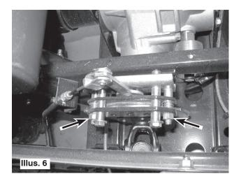
Loosen the two brake caliper bolts (C) in equal increments. Remove the bolts from the frame and lift park brake assembly out.
