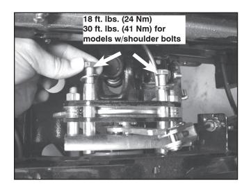
8. Install the cable, pin, and clip pin. Illus. 4 the park brake for proper function.
