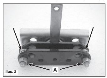
3. Slide the brake pads and springs from the assembly.
