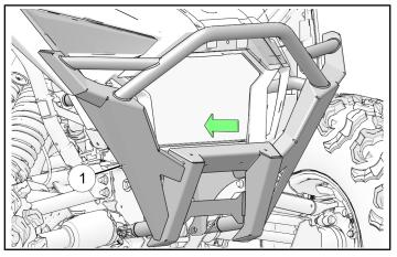
2. Install bumper ① onto fascia support bracket ② with two screws ⑤.
