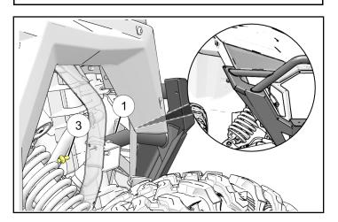
4. Install each lower-arm of bumper ① with one screw ④ and one nut ⑥.
