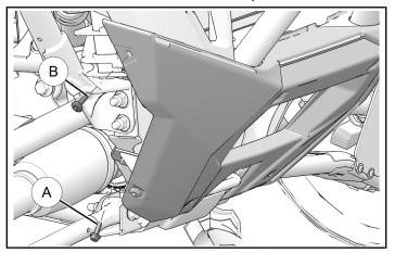
2. Reinstall one screw (B) to secure front fascia to cooling shroud.
