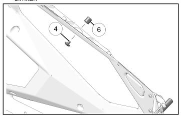
3. From inside of door, torque two shorter fasteners4 and four longer fasteners 3 to specification.
