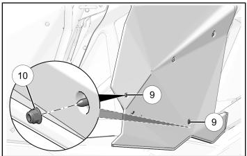
7. Install one spacer ① between door frame and aluminum door with one fastener ⑧ with and one nut ⑩.
