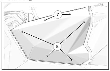
5. From outside of door, torque two shorter fasteners ① and four longer fasteners ⑧ to specification.
