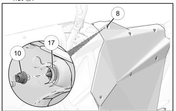
8. Counter-hold nuts (where applicable) and torque all fasteners to specification.
