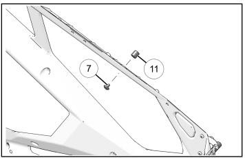
3. From inside of door, torque two shorter fasteners ① and four longer fasteners ⑧ to specification.
