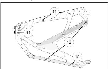
2. Install fastener and spacer combinations onto door casting. Spacer ① and fastener ② shown; others similar.
