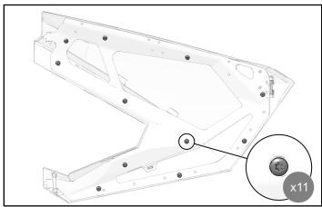
2. Remove two bracket fasteners and trim bracket from door panel.
