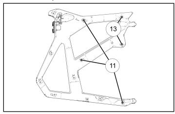
2. Install fastener and spacer combinations onto door casting. Spacer ① and fastener ⑦ shown; others similar.
