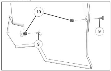
5. Align door panel with spacers and loosely install with five shorter fasteners ①.
