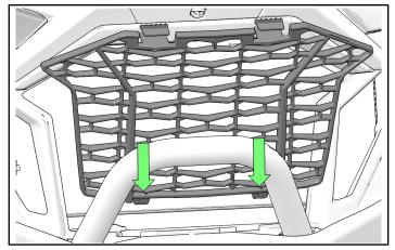
2. Push top of grille into front fascia until two tabs engage with fascia and are secure.
