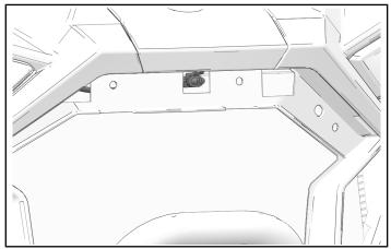
4. Align accent light ① with front fascia and secure with four speed nuts ②.
