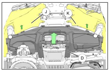
2. Ensure that tabs on panels ① and ⑥ are aligned in slots on dashboard top ⑩. (Only panel ⑥ shown. Panel ① is similar.
