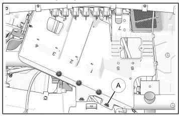
8. Reinstall audio harness to accessory mounting panel and Polaris Pulse® bar.
