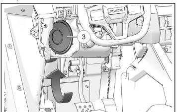
3. Loosely install speaker with two speaker fasteners§. After both fasteners are installed, torque fasteners to specification.
