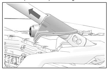
2. From underside of A-pillar cover, insert one tweeter speaker ② into tweeter cover.
