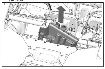
4. Install amplifier ① onto accessory mounting panel with four amplifier fasteners ⑦. Pass bottom-right fastener through ground jumper ⑤ before passing through amplifier. Ensure amplifier connector is facing downward.
