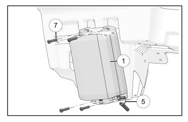
5. Return accessory mounting panel, with amplifier installed, to install position.
