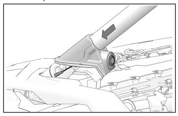
Ensure tweeter cable routes into underdashboard. Ensure A-pillar cover is completely seated into body plastic.
