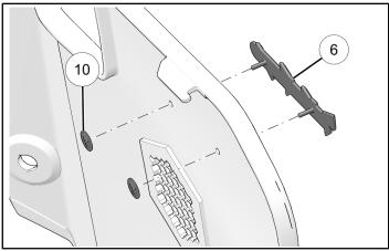
7. Reinstall speaker panel with two retained fasteners (A).
