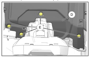
4. On front of vehicle, near rear edge of center hood panel opening, remove and retain two screws (a) from dashboard top (b). Remove and retain two pushpin rivets (h) from front side panels.
