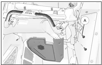
2. Tilt right-hand driver assembly ③ up-and-into installed position. Ensure driver cable routes upwards into under-dashboard.
