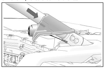
4. Ensure tweeter cable routes into underdashboard. Ensure A-pillar cover is completely seated into body plastic.
