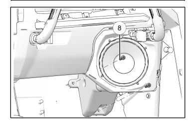
4. Install speaker to dashboard panel with four fasteners ③.
