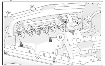
3. Maneuver accessory mounting panel from beneath Polaris Pulse® bar and remove from vehicle.
