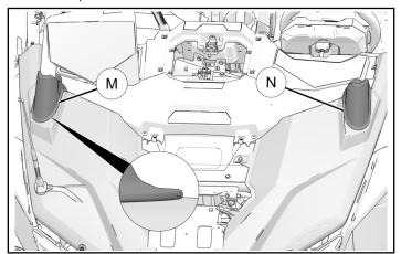
4. Reinstall two retained screws © into front edge of dashboard top ① and two retained pushpin rivets
