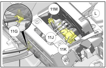
b. Secure display harness (1) to display bracket using edge clip 11M, and to bottom of chassis cross-member using routing clip 11G.
