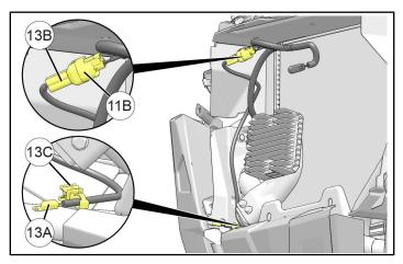
Route sensor 13A downward to prevent contact with hot components (including regulator), sharp edges, or moving parts.
