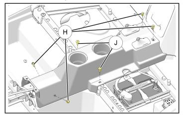
h. Remove engine access panel (located between seats).
