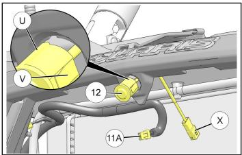
c. Remove cap from connector 11A on display harness (1), then join to connector (3) on front camera (1).
