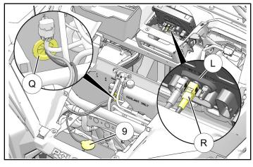
b. Route opposite end of harness to antenna mounting location on radiator shroud. Ensure routing prevents contact with hot components, sharp edges, or moving parts.
