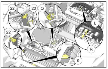
b. Route opposite end of harness to antenna mounting location on radiator shroud. Ensure routing prevents contact with hot components, sharp edges, or moving parts.
