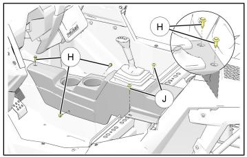
ii. Remove four push pin rivets (1) and two screws (1) from rear floor console. Remove console, pushing boots for gear shift and seat belt through console openings. Disconnect RH side auxiliary power port (if installed). Retain rivets and screws.
