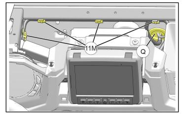
d. Secure display harness (1) to chassis support structure using four edge clips 11M.
