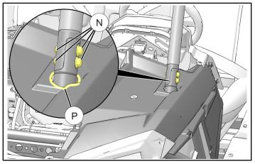
iv. Carefully lift fender over ROPS fasteners and up A-pillar, rotating as required, to gain access to upper dash structure.
