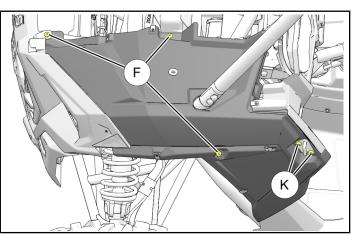
ii. Carefully pull fender from beneath front fascia at location ①. Also pull instrument panel slightly rearward, disengaging two retaining clips (1) from fender.
