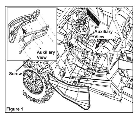
3. Mount the spacers on the door frame (PN 5139035, PN 5139036 and PN 5139037) using six M6 screws. Figure 2.
