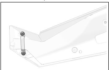
3. Remove door panel from door and carefully set aside.
