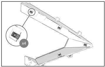
3. Install four retained U-nuts to mounting locations of accessory close-off panel.
