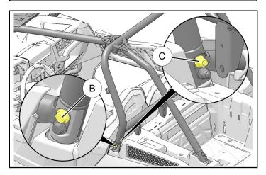
3. Loosely install strap <sup>(1)</sup> using mounting bolt <sup>(B)</sup> and nut <sup>(C)</sup>. Do not tighten bolt at this time.
