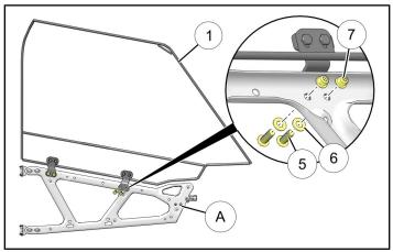
If door ① is not centered front to rear, between A-pillar and rear window, then loosen four each nuts
