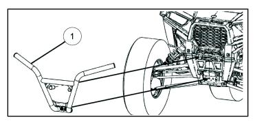
3. Ensure expansion anchors are fully seated by slowly rotating each anchor assembly ③ ④ ⑤ ⑥, verifying that flat faces of tube ⑤ have slipped into and aligned with flat faces of welded socket ④ as shown.
