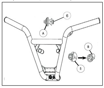
4. Using arc-joint pliers, grasp expansion tube ⑤ and remove from frame at each attach point. During removal tabs will straighten as shown by ⑧ above. Discard old hardware.
