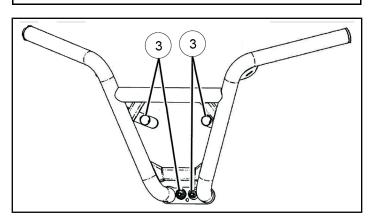
5. Insert two plugs ② into bumper as shown.
