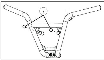
6. Insert two plugs ① into outboard ends of bumper tubing (if not pre-installed from factory).
