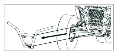
3. Using pin punch, drive wedge (a) rearward out of expansion tube (5) at each attach point as shown.
