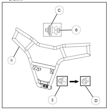
4. Using arc-joint pliers, grasp expansion tube ⑤ and remove from frame at each attach point. During removal tabs will straighten as shown by ⑩ above. Discard old hardware.
