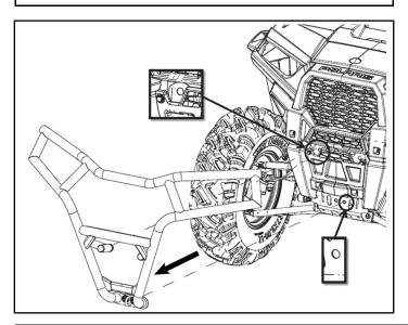
3. Using pin punch, drive wedge **(6)** through expansion tube into frame at each attach point as shown.
