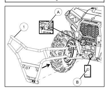
3. Ensure expansion anchors are fully seated by slowly rotating each anchor assembly ③ ④ ⑤ ⑥, verifying that flat faces of tube ⑤ have slipped into and aligned with flat faces of welded socket ⓒ as shown.
