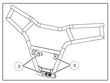
5. Insert two plugs ② into bumper as shown.
