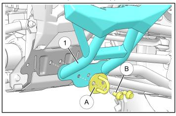
5. Torque screws to specification.
