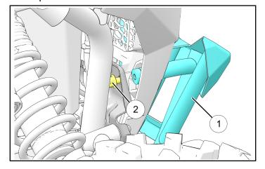
4. Loosely install two retained screws ® through tow hook (a) and bumper ① into support plate.
