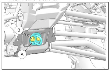
3. Loosely install screw ② through LH side of front suspension mounting bracket into bumper ①. Repeat for RH side.
