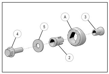
4. While ensuring upper portion of bumper is firmly seated against vehicle frame, and flats are properly aligned, tighten two upper screws ④ and washers ⑤. Torque to specification.
