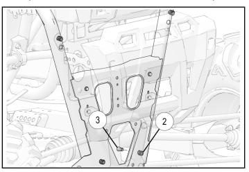
3. Using arc-joint pliers, grasp expansion tube ② and remove from frame at each attach point. Discard old hardware.
