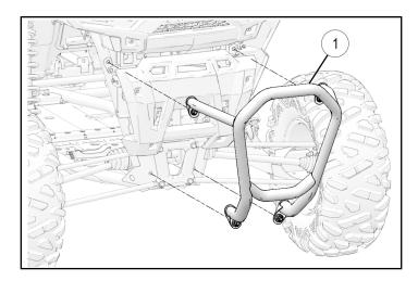
3. Ensure expansion anchors are fully seated by slowly rotating each screw 4 until flat faces of expansion tubes 2 slip into and align with flat faces of bumper bracket (A) as shown.
