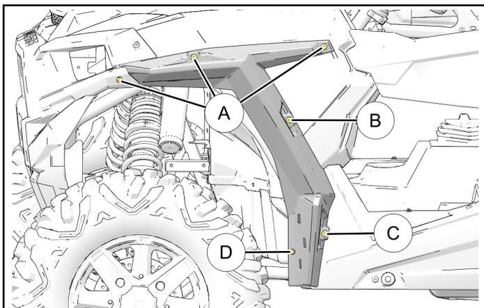
3. Install new LH fender (1) using retained screws (A) (B) (C), and one plastic push pin (D) as shown.
