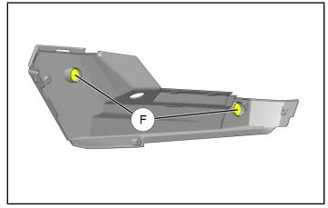
4. Remove plug 6 from interior LH side of floor pan.
