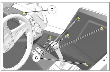
c. From outside of vehicle, and while supporting exterior body panel, remove final screw ①, then remove panel by detaching locking tab ① from mating slot in front fender. Set panel aside.
