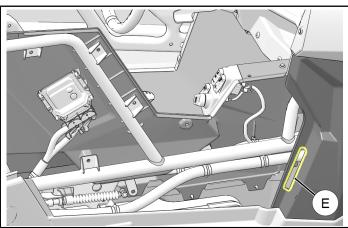
Use 1–3/4 inch (44 mm) hole saw to cut two openings in LH rocker panel at marked locations
