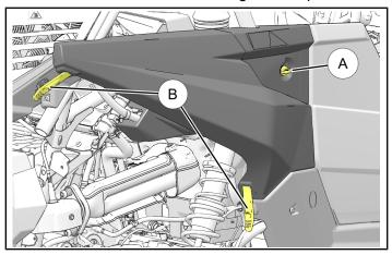
b. Remove five screws © securing RH exterior body panel to frame. Retain screws.
