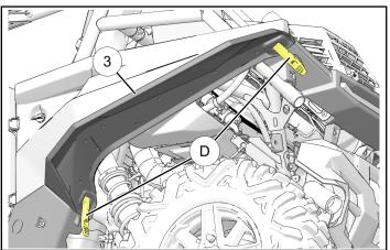
b. Lift and hold bumper in final position, then using fender as template mark nine fastener holes (£).
