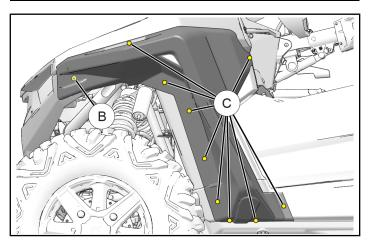
c. Remove fender ① from vehicle, then drill nine 5/16 inch (8 mm) holes through vehicle body panels at marked locations ©.
