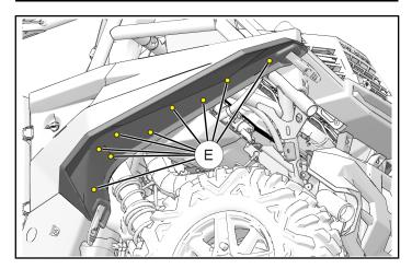
c. Remove fender ③ from vehicle, then drill nine 5/16 inch (8 mm) holes through vehicle body panels at marked locations ⑤.
