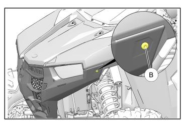
b. Loosely install left front fender ① to vehicle using retained screw ®, hold rear side of bumper in final position, then using fender as template mark nine fastener holes ©.
