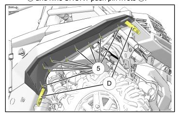
e. Repeat Steps a-d on RH side of vehicle using right rear fender ④.
