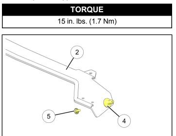
d. Install clamp (6) to windshield visor (2) using two screws (7) as shown. Ensure proper orientation: Clamp latch tab is on OUTBOARD side of visor. Torque to specification. Repeat for opposite side.
