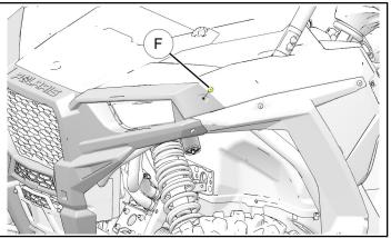
b. Install screw (5) and shoulder spacer (6) into front fascia as shown. Repeat for RH fender.
