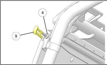
f. Center windshield in ROPS, push fixed portion of windshield ① down against upper dash panel to compress seal, then tighten nuts <sup>(1)</sup>. See Step 4d for illustration. Torque to specification.
