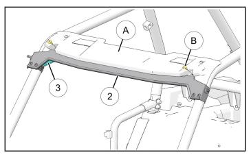
g. Using fingers, squeeze clamp straps together until they lock.
