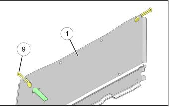
c. Install LH bracket <sup>(1)</sup> to fixed (lower) portion of windshield <sup>(1)</sup> using two push darts <sup>(2)</sup> as shown. Repeat for RH bracket <sup>(1)</sup>.
