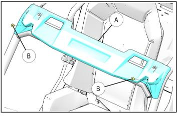
b. Orient seal 3 so bulb is facing forward/upward, then install to ROPS visor (A) by pushing into place as shown. Trim seal to fit (if necessary).
