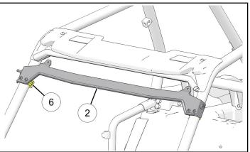
f. Align fastener holes, then loosely install windshield visor ② to ROPS visor (A) using two retained screws (B) as shown.
