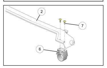
e. Open clamps (6), then push windshield visor (2) onto ROPS A-pillars as shown.
