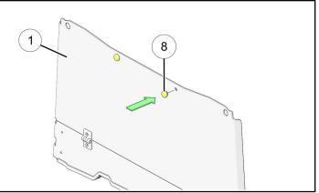
b. Install two straps (1) to windshield (1) by pushing straps through BACK side of windshield as shown.
