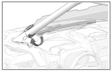
Windshield may need repositioning. If needed, release clamps and slide windshield up along ROPS.
