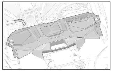
3. With windshield in correct position, secure to ROPS with two Lock & Ride<sup>®</sup> clamps.
