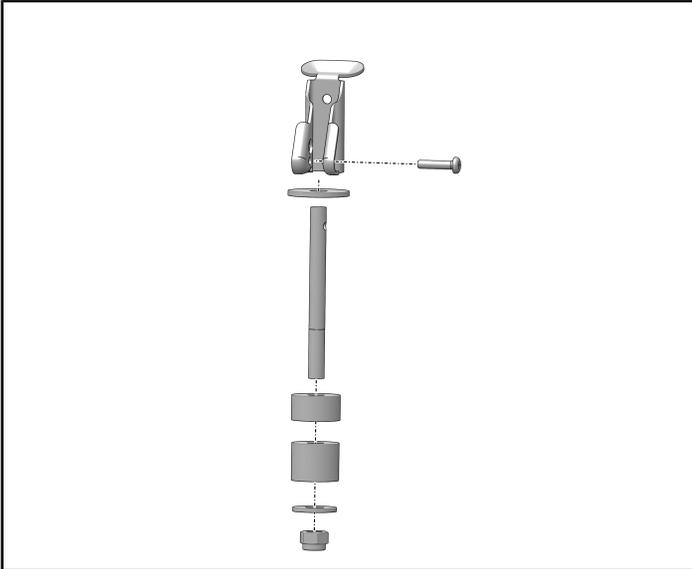
3. Install lock and ride anchors ③ on to the cargo box.
