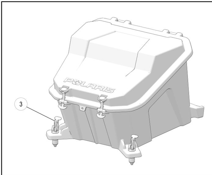
4. Slide the box on the vehicle so that storage box base ⑤ protrusions on the box are seated into the slot on the body.
