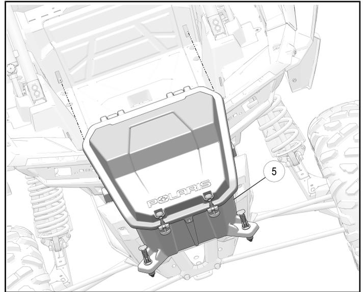
5. Install the storage box base ⑤ onto the vehicle body.
