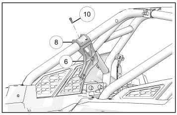
2. Position pivot bracket assembly at specified location.
