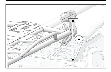
Install each post clamp onto ROPS with clamp bracket ③, two clamp fasteners ④, and two clamp nuts ⑬. Ensure latch plunger aligns with tire rack, as shown.
