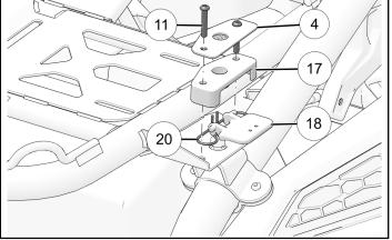
11. Ensure spare tire rack comes into contact with rubber bumpers on both sides. Inconsistent contact may result in one or two dysfunctional latches.
