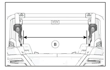
5. Install one strut (19) on each side. Note orientation of strut in graphic below.
