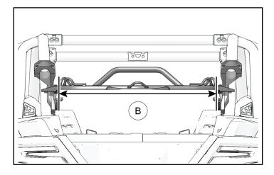
8. Verify assembly positioning before torquing pivot bracket fasteners.
