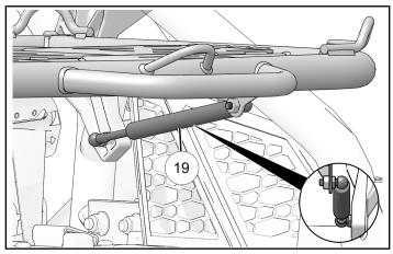
Position tire rack in rear cargo box and pass pin (5) through pivot bracket, bushing (4) (two passenger vehicles only), and thread into tire rack.
