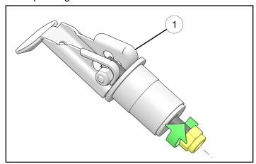
4. Ensure Lock & Ride® assemblies ① are fully seated before closing top lever and securing storage box.
