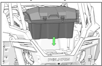
2. Place four Lock & Ride® assemblies ① in four aligned mounting holes.
