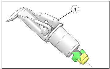
5. Ensure Lock & Ride<sup>®</sup> assemblies ① are fully seated before closing top lever and securing storage box.
