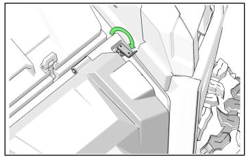
7. Reinstall Lock & Ride<sup>®</sup> assemblies into rear storage box.
