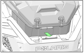
3. Place two Lock & Ride<sup>®</sup> assemblies in two aligned mounting holes.
