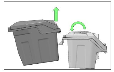
3. Ensure front protrusion of storage box hooks under rear box tube.
