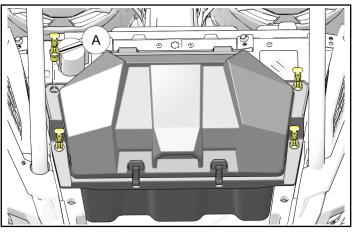
2. Lift front storage box up slightly to allow rear storage box protrusion to fit below front storage box lip as shown.
