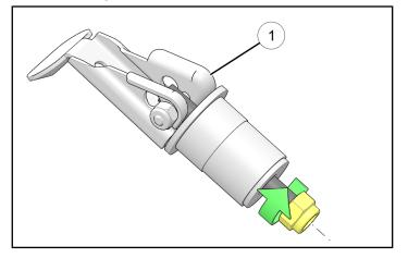
6. Ensure Lock & Ride<sup>®</sup> assemblies ① are fully seated before closing top lever and securing storage box.
