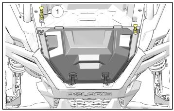
4. Lock & Ride<sup>®</sup> assemblies ① may need adjustment. Tighten or loosen bottom nut depending on fitment.
