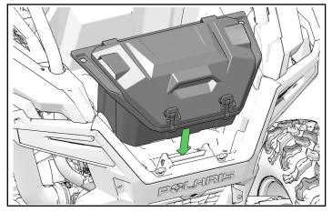
2. Ensure front protrusion of storage box hooks under rear box tube.
