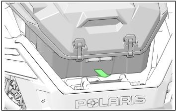
4. Place two Lock & Ride<sup>®</sup> assemblies in two aligned mounting holes.
